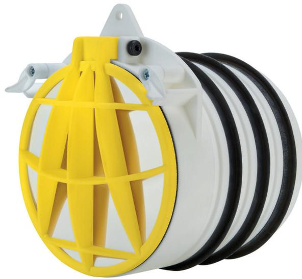
The 150mm/6" Buffalo Valve offers a robust solution for protection against sewage back water, vermin and insects. This easy to install non-return valve can be retro fit to any clay or plastic 150mm 6inch pipe. The Buffalo valve also includes a steel reinforced plate to guard against pests such as rats and snakes, and a lockable flap to allow for essential maintenance.
